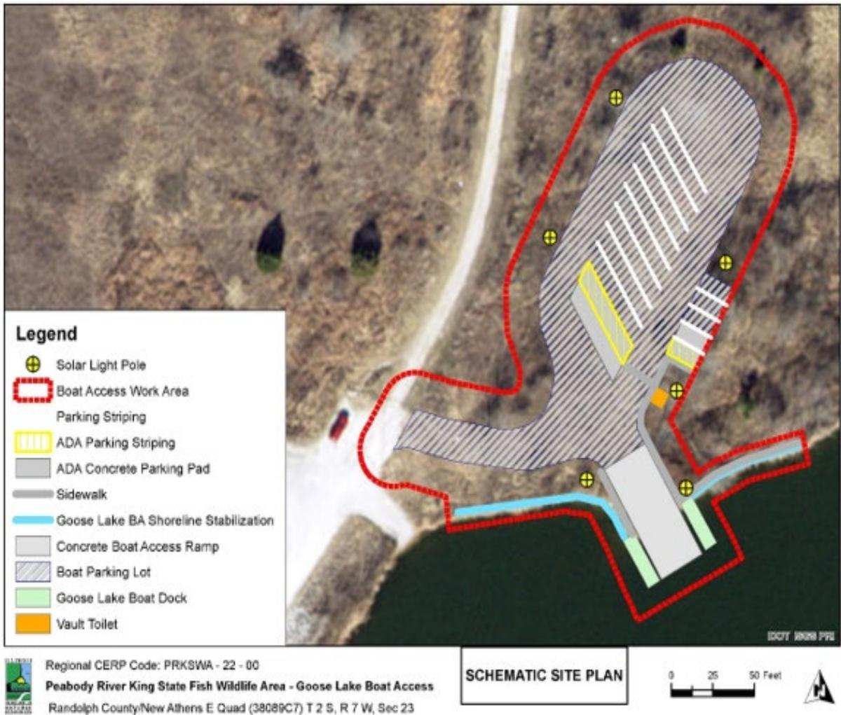
*Example Small Access Schematic Site Plan*
